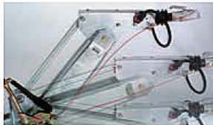
Height-adjustable drawbar (ball head coupling and DIN towing eye not included)
