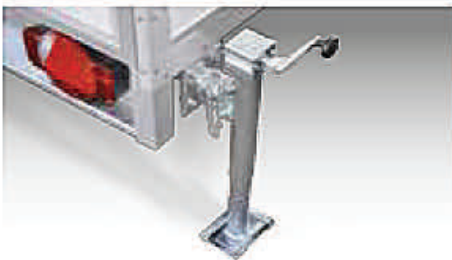
Telescopic crank supports for box trailers (2 x)
